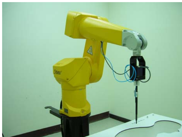
Fig. 5.2 Probe setup on robot
