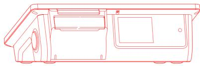
Insert the thermal paper and pull out part of it outside the paper exit of the printer, then close the paper compartment cover;
