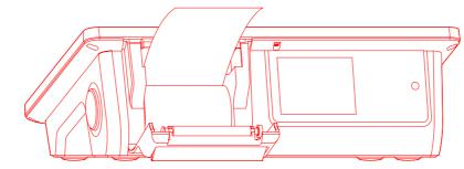
After printing, tear the paper upwards.
