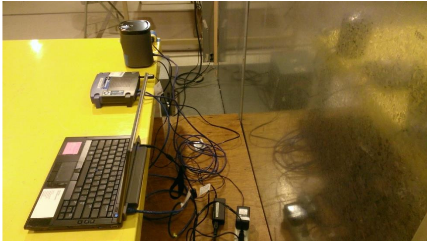
LINE CONDUCTED BACK PHOTO
