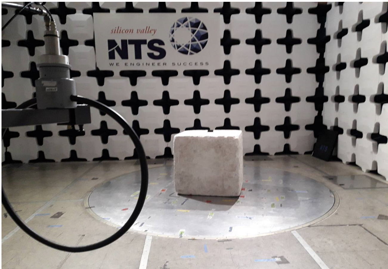
Test Configuration Photograph #1 (Radiated Emissions - Below 30 MHz)
