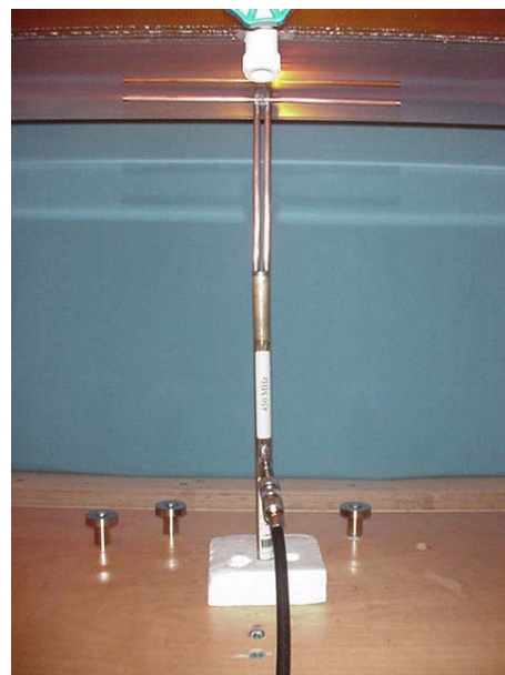
450 MHz Dipole Setup
