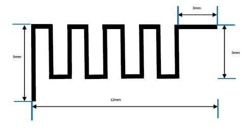
Since there is no ground plane beneath the antenna, PCB thickness will have little effect on the performance. The results presented in this design note are based on an antenna implemented on a PCB with 1 mm thickness.
