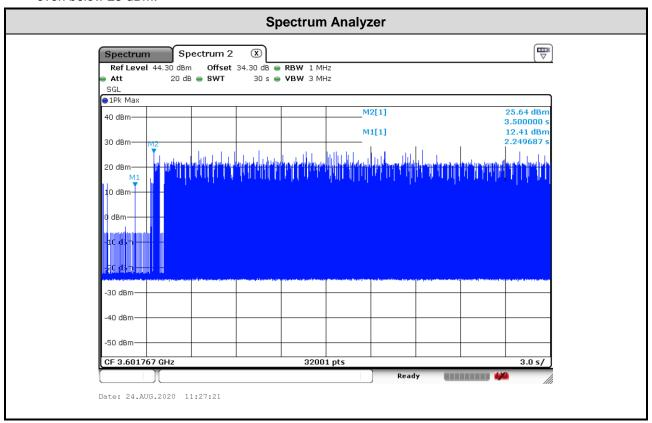
Note: The Ref Offset 34.3 dB includes the antenna gain 16 dBi and cable path loss 18.3 dB.
