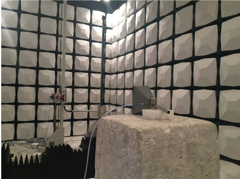
Description: Substitution Antenna for EIRP Test
