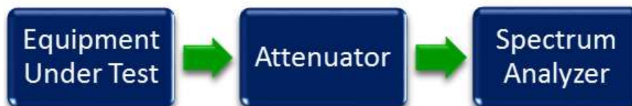
Figure 3: Spurious Emission at Antenna Terminal Test setup
