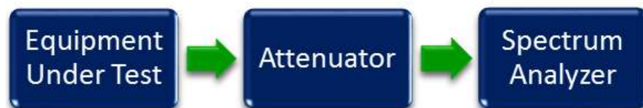
Figure 1 Output RF power Test Setup
