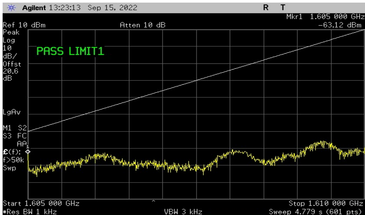
Plot 24-High Channel – Test Limit 25.216 (f)(g) – Discrete Emissions
