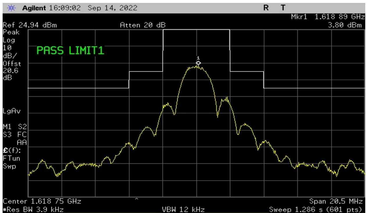
Plot 6 – Emission Mask - High Channel
