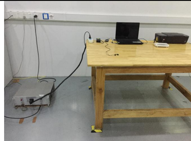
Conducted Emissions Test Setup – Front View
