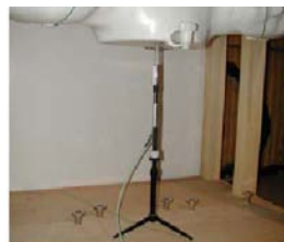
Figure 11.1 Dipole Verification Test Setup Diagram & Photo
