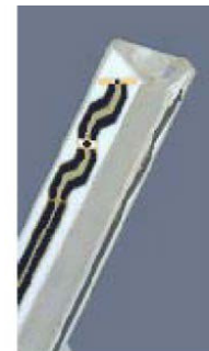
Figure 3.3 Probe Thick-Film Technique
