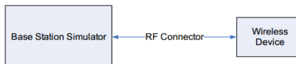
Figure 10.1 Power Measurement Setup
