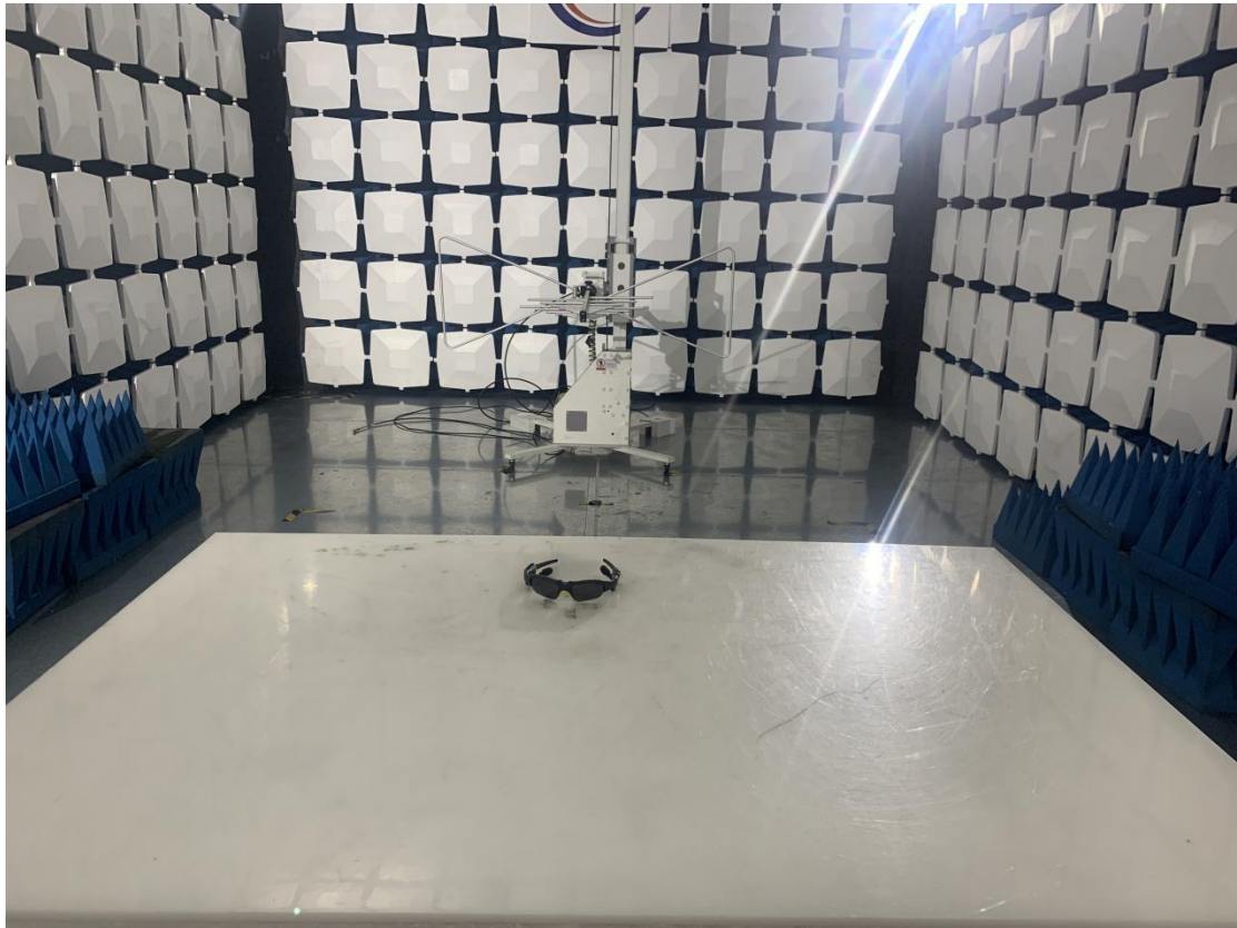
Below 1GHz for radiated emission test setup
