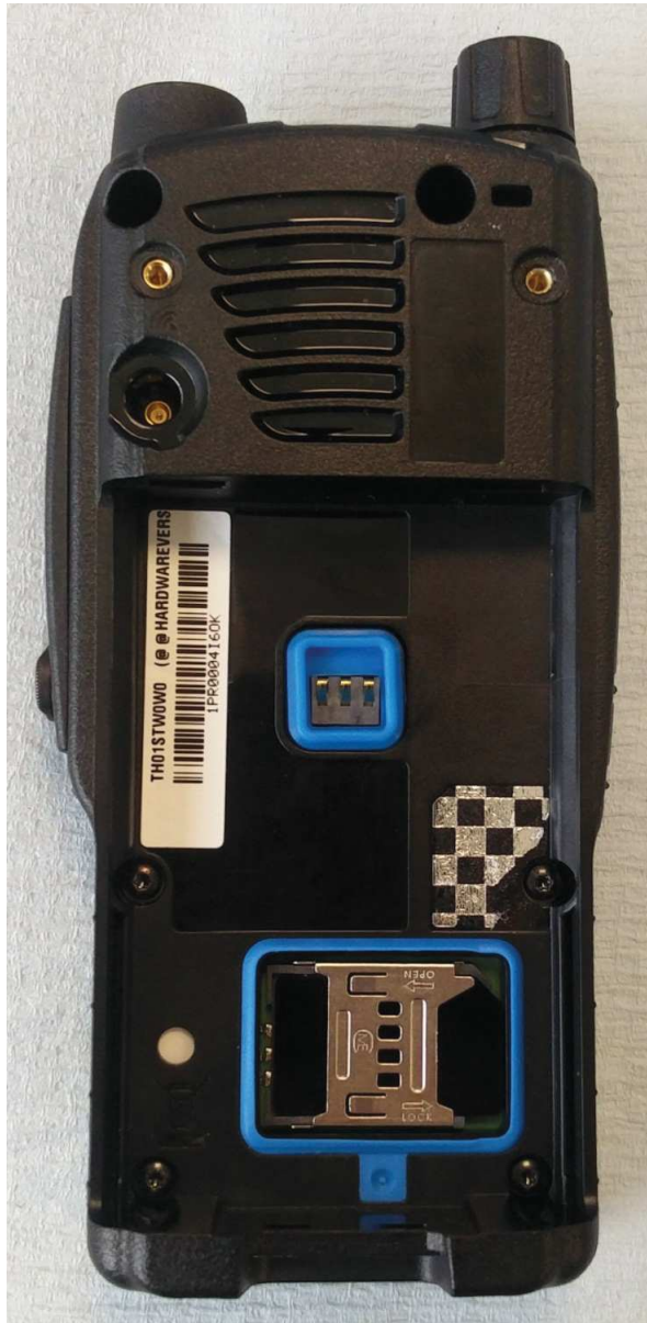
Figure 3. XX6SC2128 Rear with Battery and Antenna Removed
