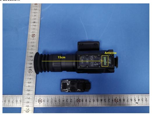
Minimum distance from antenna to eyepiece (Head): 15cm Minimum distance from antenna to casing (Extremity): 0.5cm
