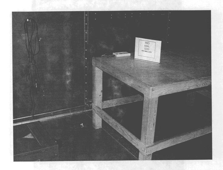
Part 3.3 Radiated Emissions Setup - Front View - 3 quantum of the best of the
