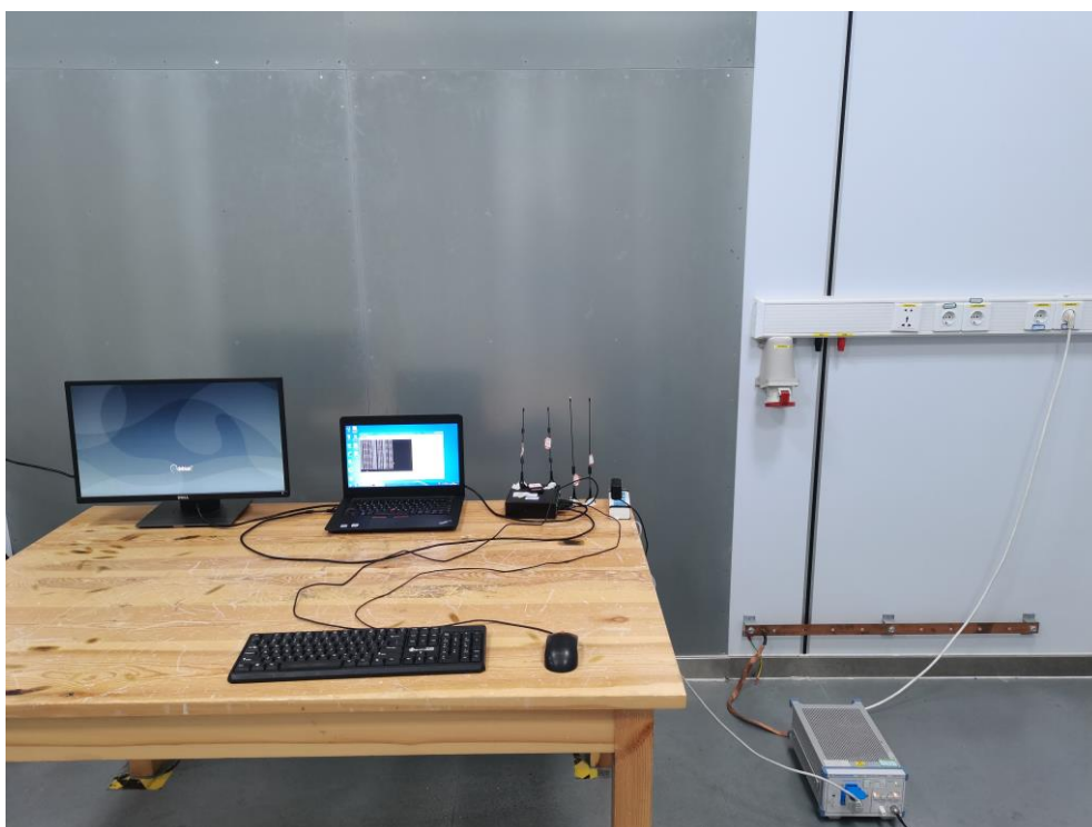
Fig. 4 Power line conducted emission setup photo
