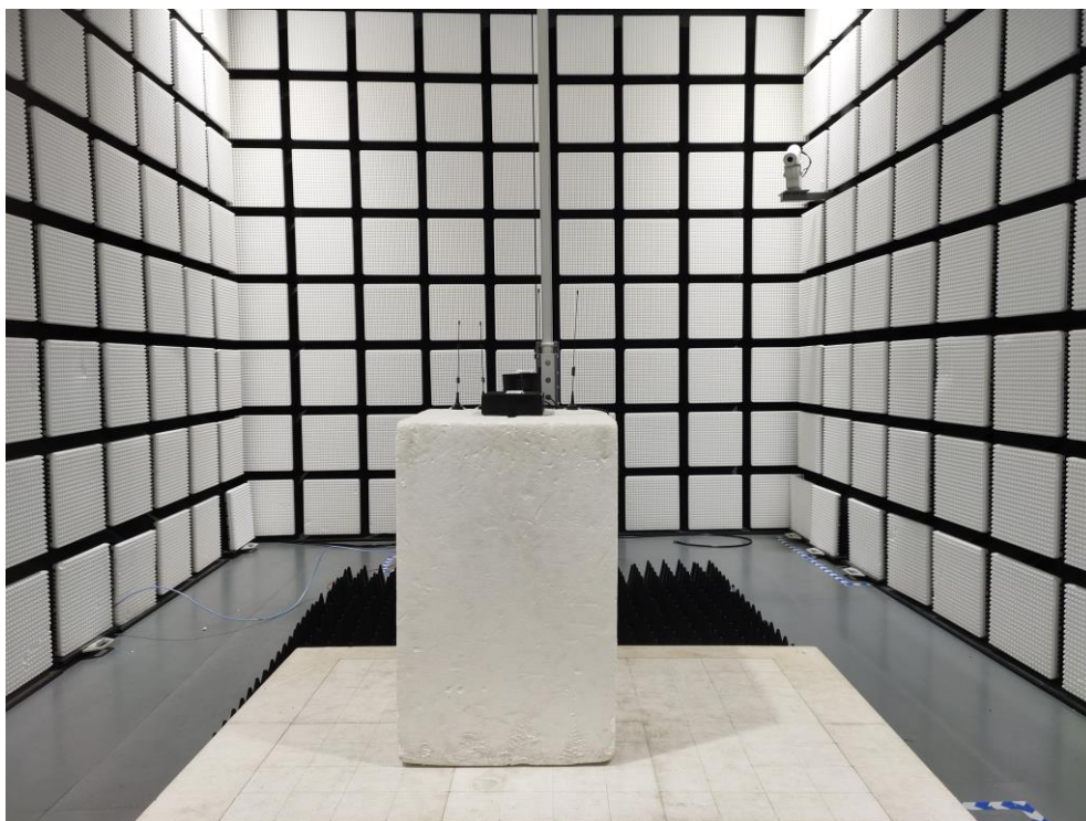
Fig. 3 Radiated emission setup photo(Above 1GHz)
