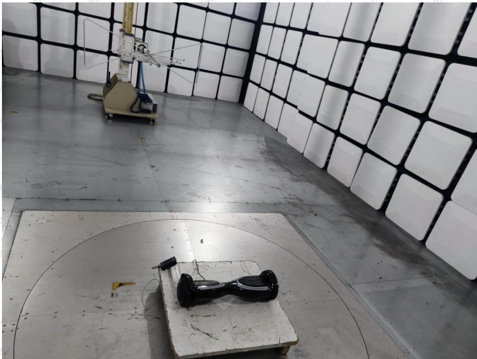
Photo of Radiation Emission Test
