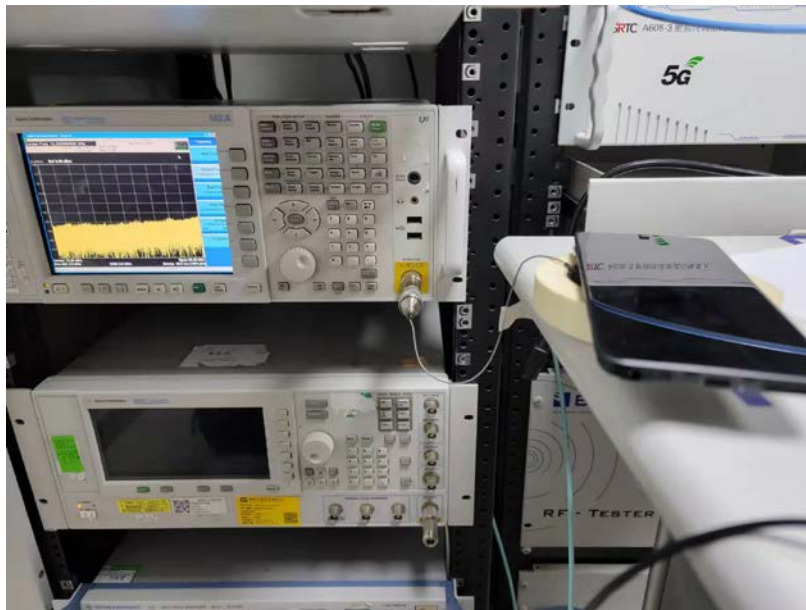
RF Conducted Test setup (BT/WIFI)
