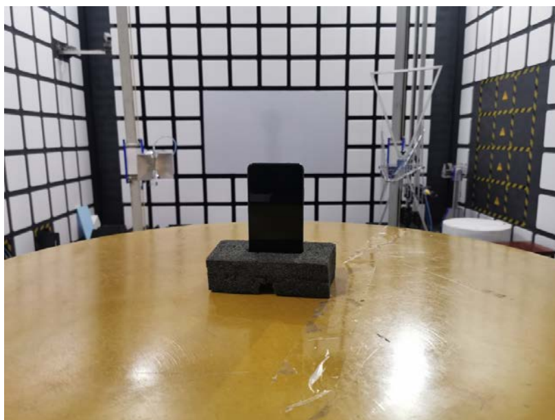
Spurious Radiated Emissions Test setup
