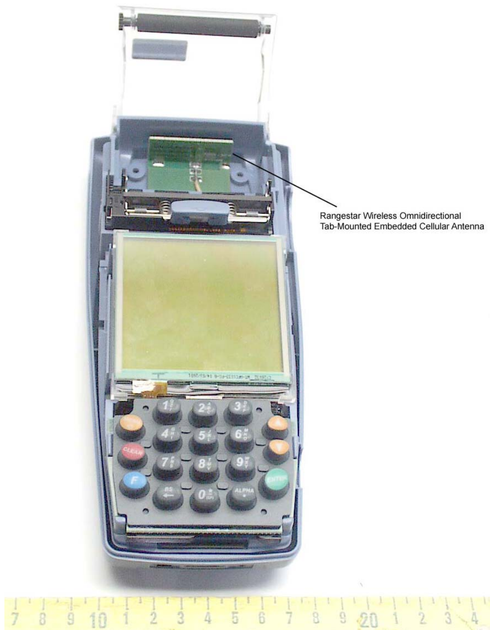
<Front View – Showing Internal Integral Antenna>
