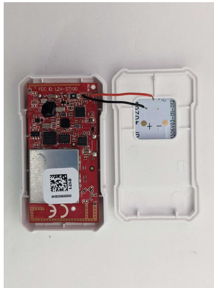
Component Side ST100 w/ wires to Solar Panel mounted in Top Housing
