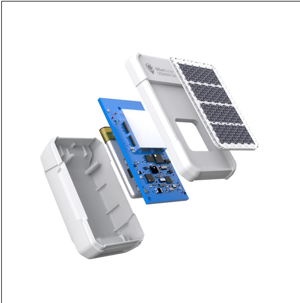
GSatSolar Exploded Internal View Drawing
