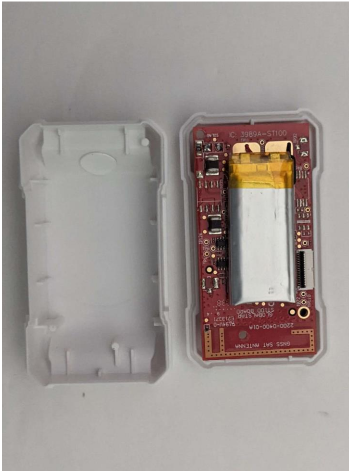
Bottom Housing / Battery mounted to Batt side ST100
