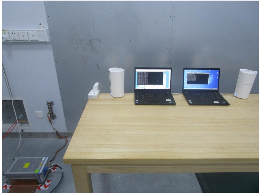
POWERLINE CONDUCTED EMISSIONS MEASUREMENT SETUP
