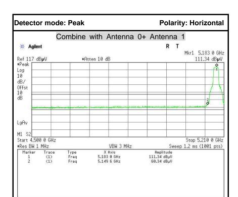
**Polarity: Horizontal** Detector mode: Average Combine with Antenna 0+ Antenna 1 R Agilent Mkr1 5.180 9 GHz 94.33 dB**µ**V Ref 117 dBpV #Atten 10 dB #Peak Log 10 dB/ Offst 10 dΒ LgAv M1 S2 Start 4.500 0 GHz Stop 5.210 0 GHz Sweep 55.36 s (1001 pts) #Res BW 1 MHz #VBW 10 Hz Trace (1) (1) Type Freq Freq X Axis 5.180 9 GHz 5.149 6 GHz Amplitude 94.33 dBμV 46.95 dBμV Marker
