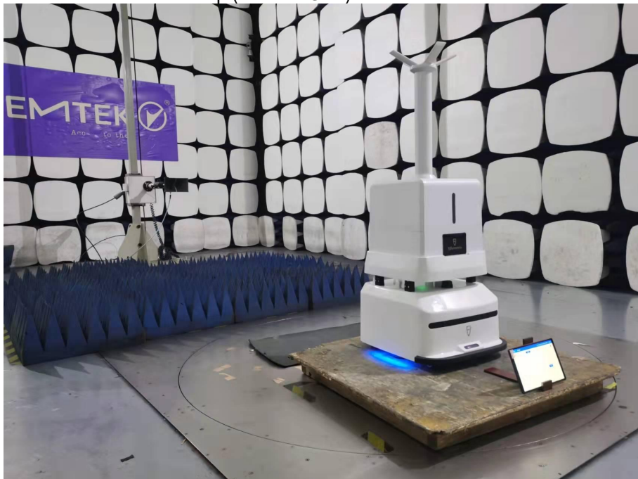
Spurious Emission Test Setup (Above 1GHz)
