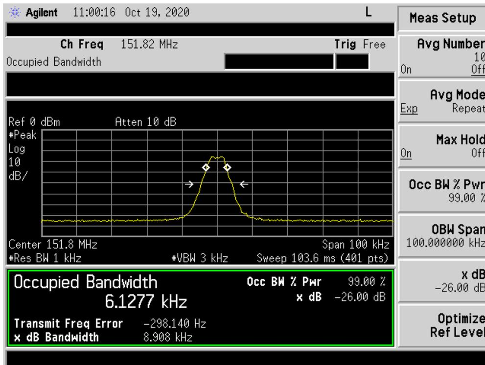
Figure 4. Bandwidth Measurement
