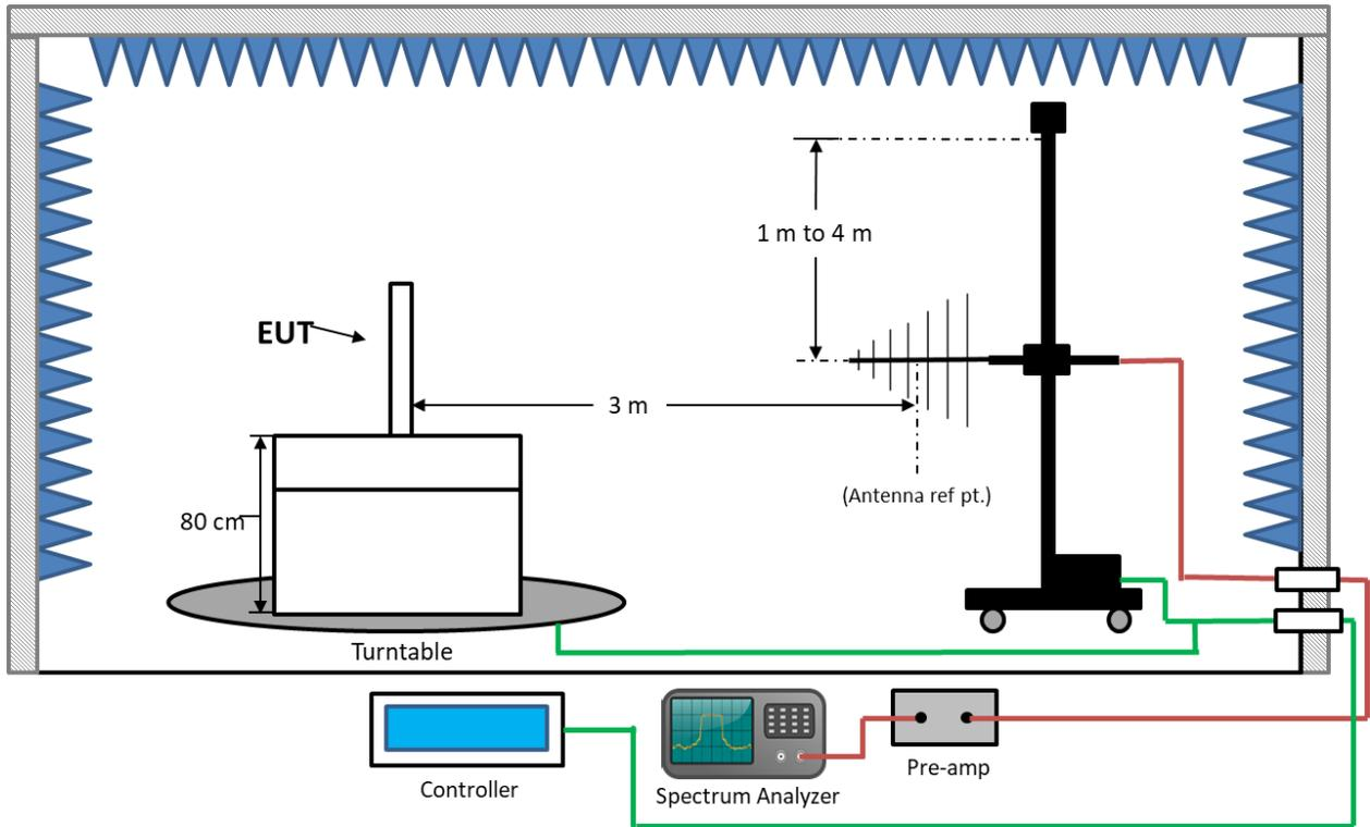
**Figure 2. EUT Test Configuration – Radiated Emissions**
