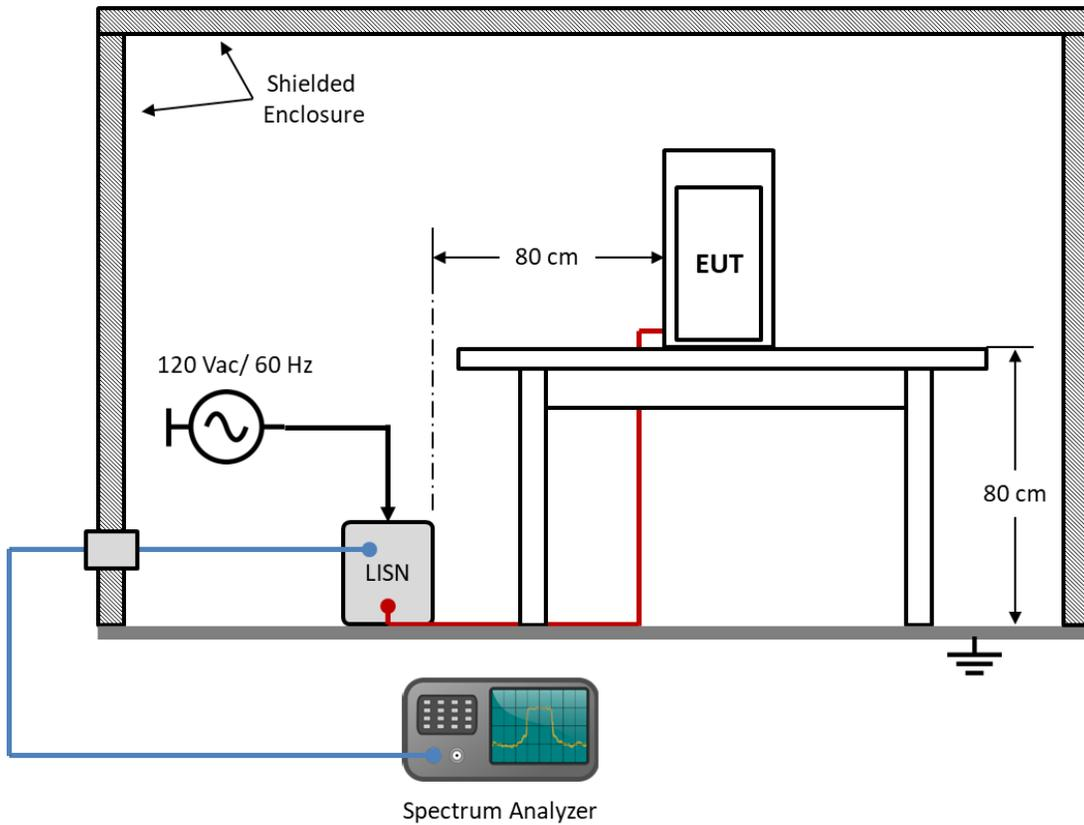
**Figure 3. EUT Test Configuration - AC Power Line Conducted Emissions**
