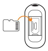
Before turning on your camera, insert a Micro SD memory card (NOT included) into the **memory card slot** ②. The memory card is needed in order to store photos or videos.
