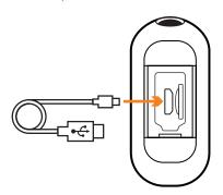
1. Insert the Micro USB end of the included USB cable into the Micro USB port © on your camera.
