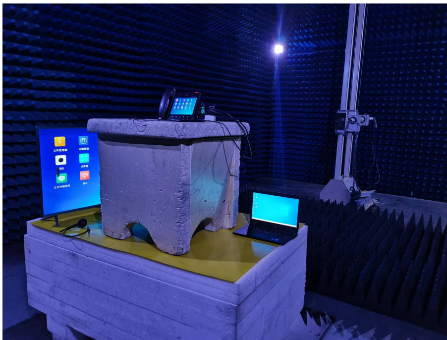
Photo of Radiated Emission Measurement (Above 1G)
