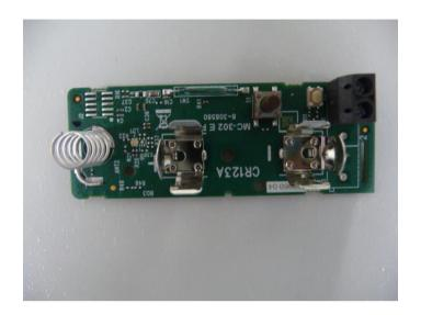
Photograph No.3 MC-302E magnetic contact PCB rear side view
