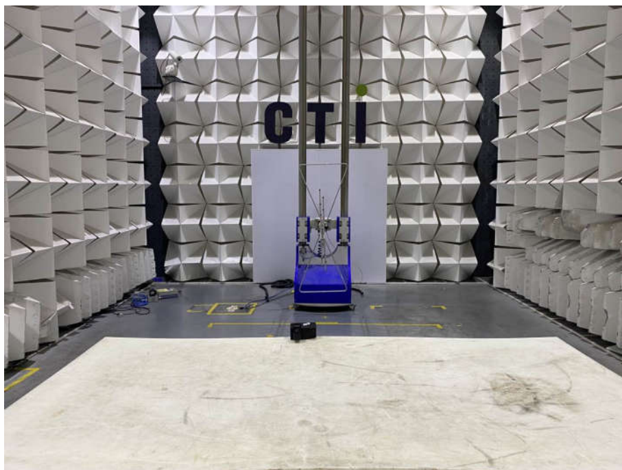
Radiated spurious emission Test Setup-1(Below 1GHz)
