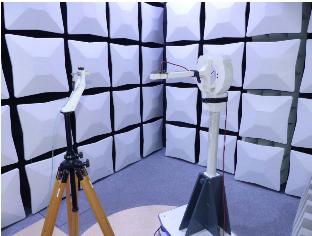
Photo 6: Test setup for radiated measurements (above 26 GHz)
