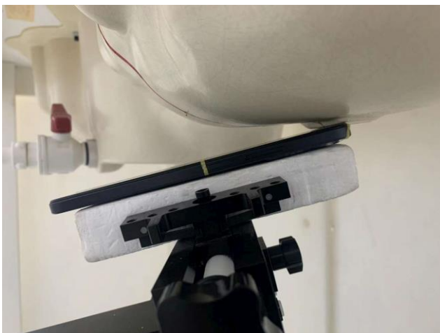
Left Tilted, Test Separation 0 mm
