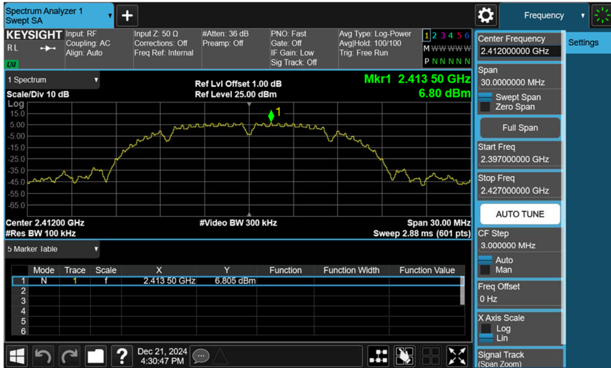
Figure 55: Conducted Spurious Emission & Authorized-band band-edge, 802.11b, 2412MHz Carrier Level
