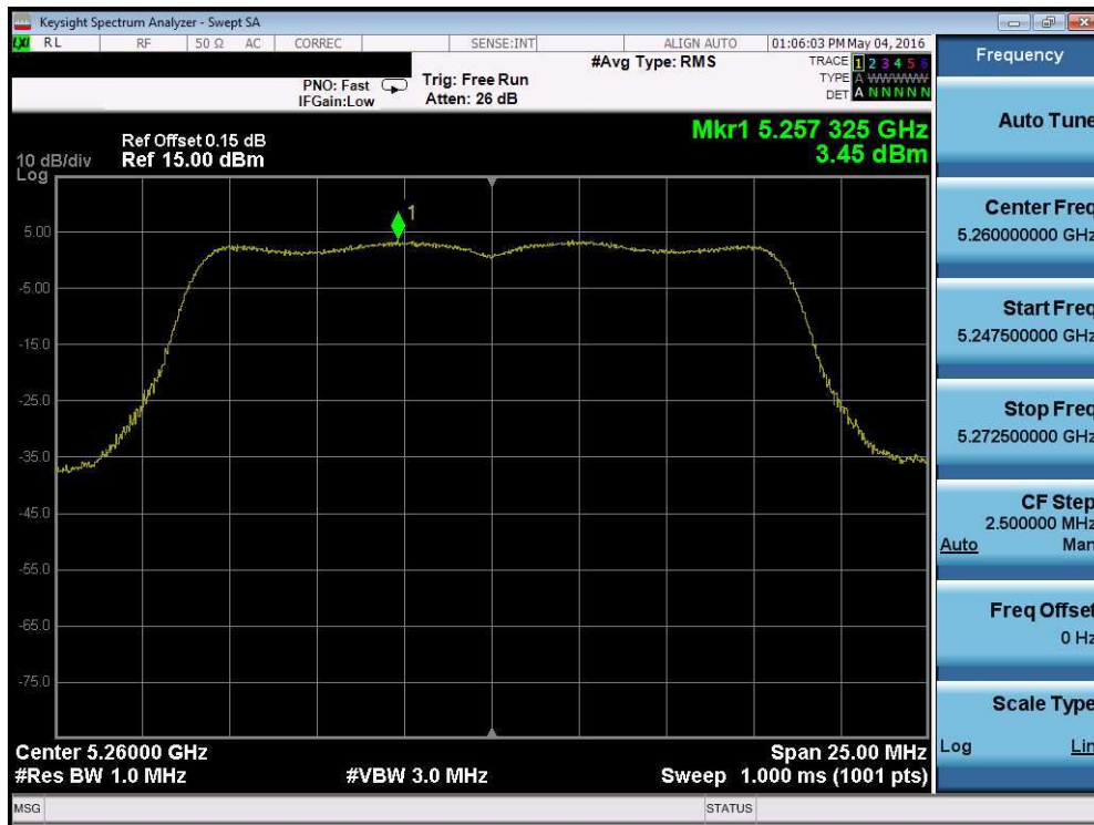
Plot 7-48. Power Spectral Density Plot (802.11a (UNII Band 2A) – Ch. 52)
