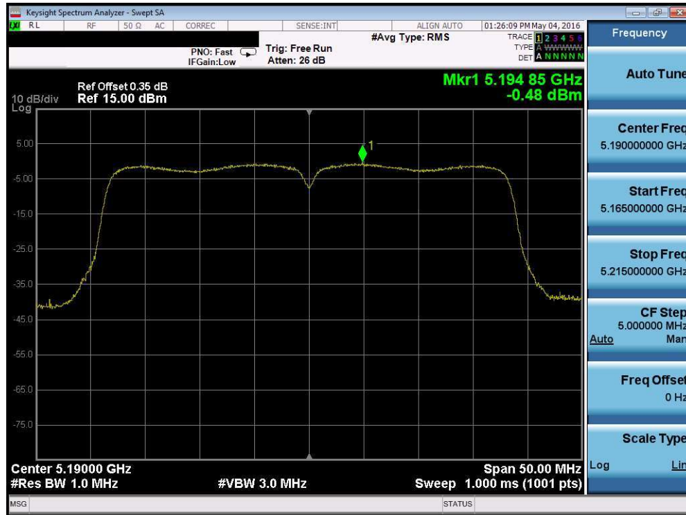
Plot 7-45. Power Spectral Density Plot (40MHz BW 802.11n (UNII Band 1) – Ch. 38)
