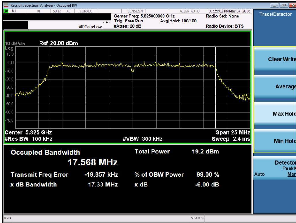
Plot 7-35. 6dB Bandwidth Plot (20MHz BW 802.11n (UNII Band 3) – Ch. 165)
