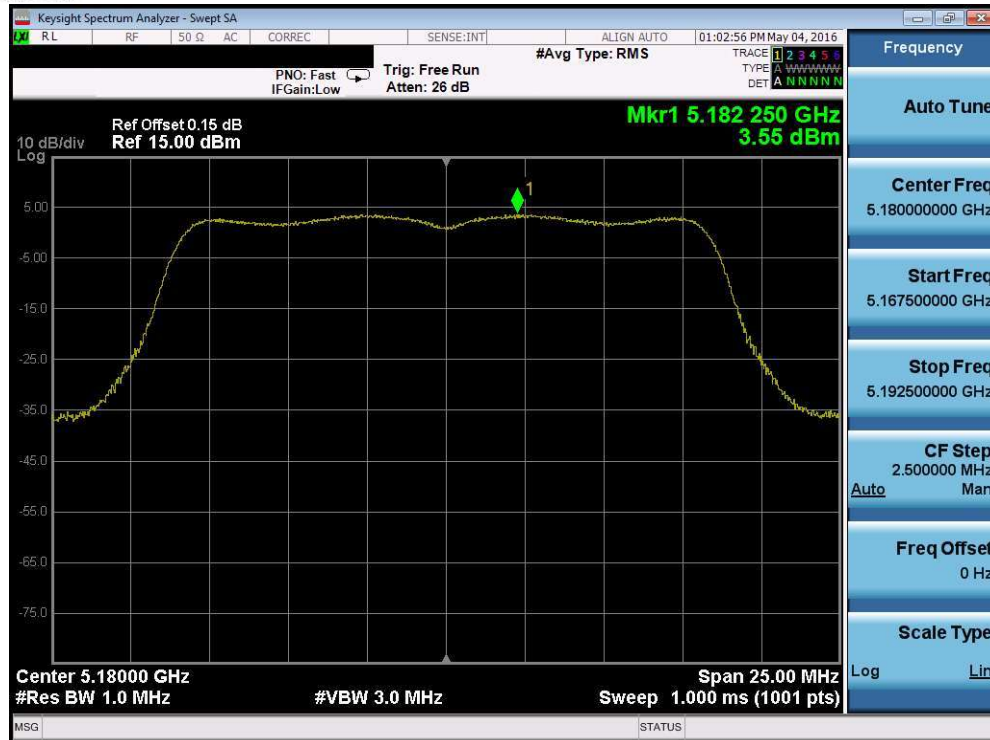
Plot 7-39. Power Spectral Density Plot (802.11a (UNII Band 1) – Ch. 36)
