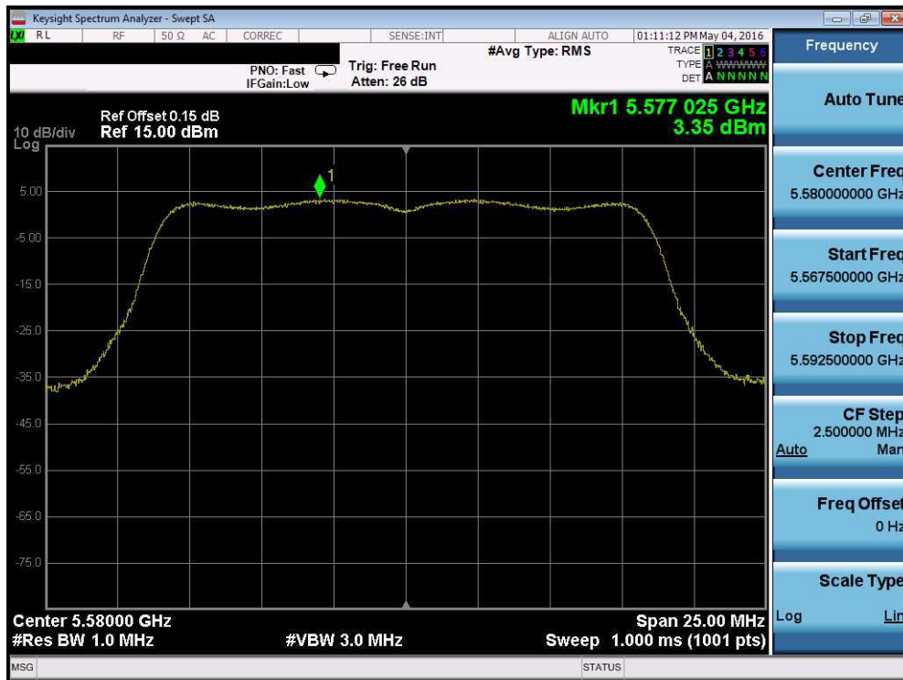
Plot 7-58. Power Spectral Density Plot (802.11a (UNII Band 2C) – Ch. 116)
