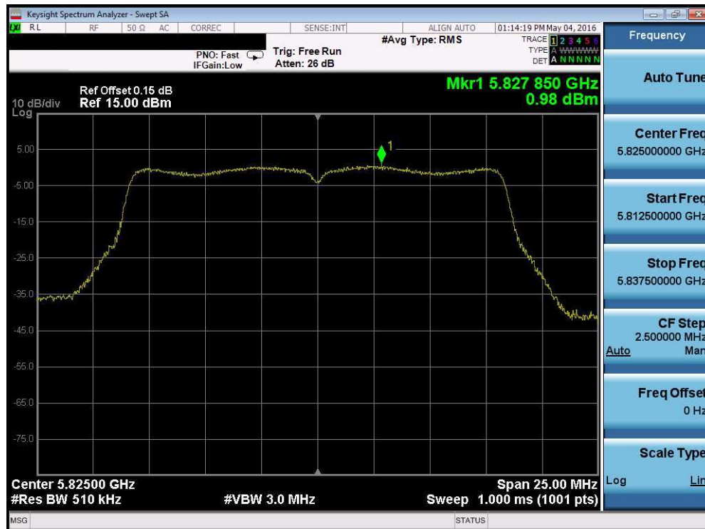
Plot 7-70. Power Spectral Density Plot (802.11a (UNII Band 3) – Ch. 165)
