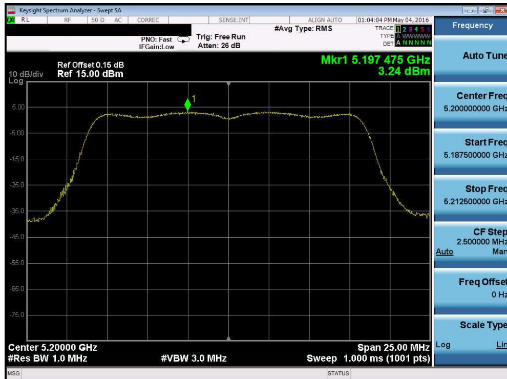
Plot 7-40. Power Spectral Density Plot (802.11a (UNII Band 1) – Ch. 40)
