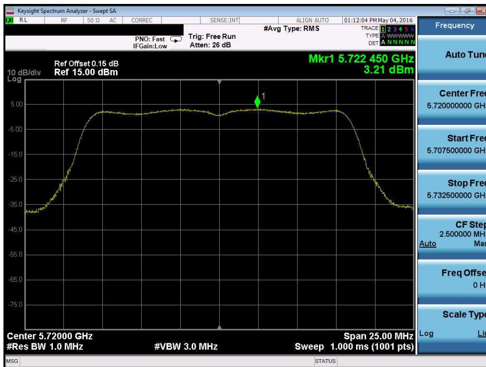
Plot 7-59. Power Spectral Density Plot (802.11a (UNII Band 2C) - Ch. 144)
