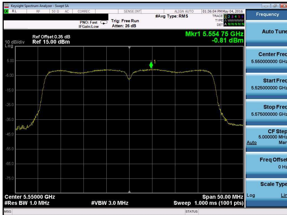
Plot 7-64. Power Spectral Density Plot (40MHz BW 802.11n (UNII Band 2C) – Ch. 110)
