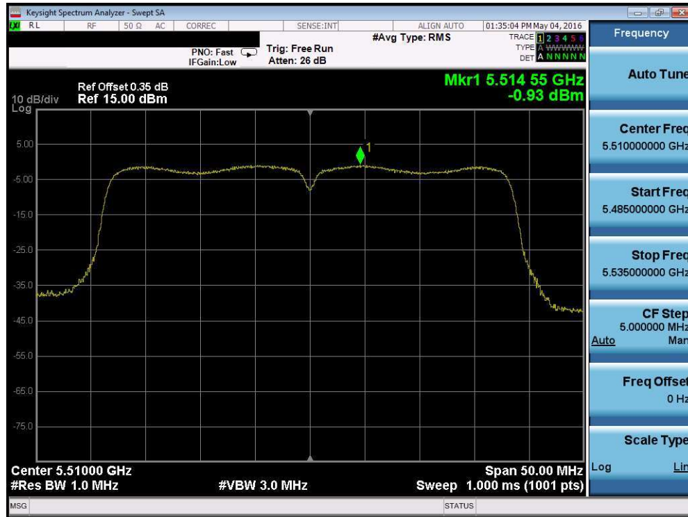
Plot 7-63. Power Spectral Density Plot (40MHz BW 802.11n (UNII Band 2C) – Ch. 102)
