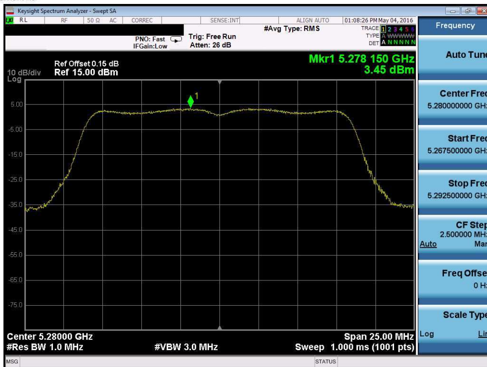
Plot 7-49. Power Spectral Density Plot (802.11a (UNII Band 2A) – Ch. 56)
