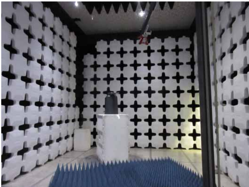
Test Setup for Spurious Emissions – 1 to 10GHz, Vertical Polarization
