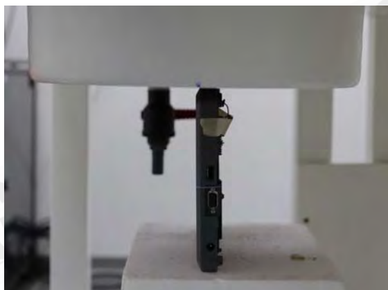
Fig.5 EUT Top side to flat phantom
