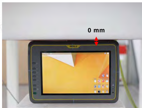
Fig.9 EUT Bottom side to flat phantom
