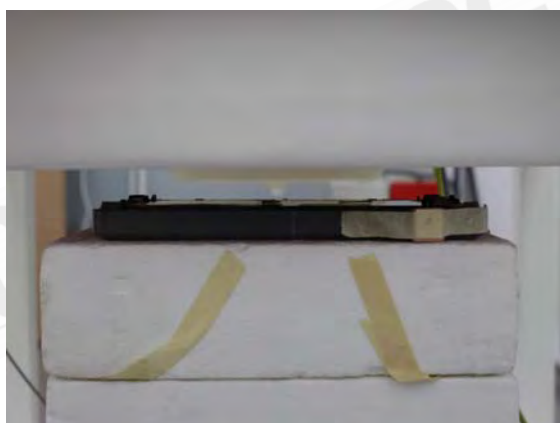
Fig.4 EUT Back side (25mm) to flat phantom
