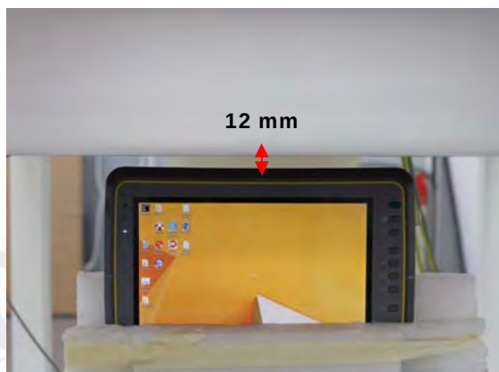
Fig.6 EUT Top side (12mm) to flat phantom
