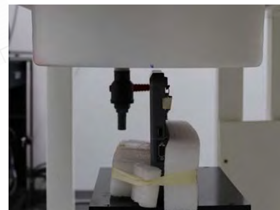
Fig.6 EUT Top side (12mm) to flat phantom
