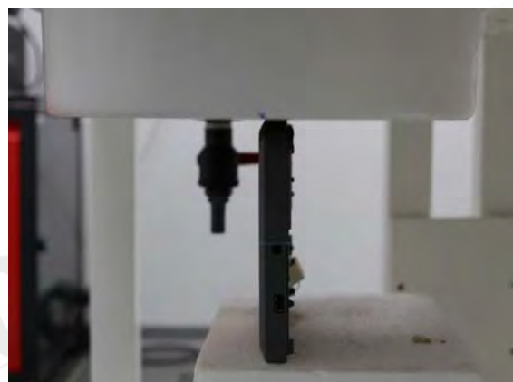
Fig.9 EUT Bottom side to flat phantom
