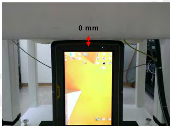
Fig.12 EUT Left side to flat phantom
