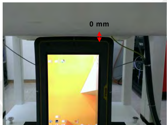
Fig.13 EUT Right side to flat phantom
