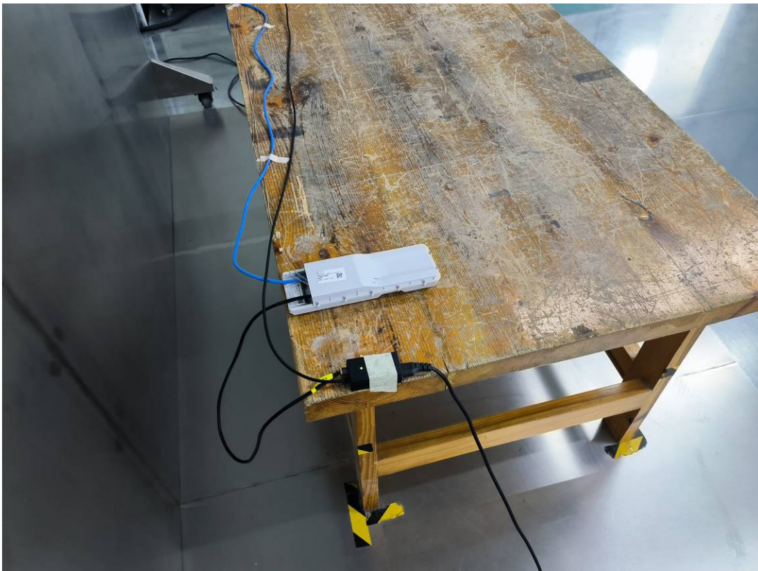
Conducted Emissions Side View POE
