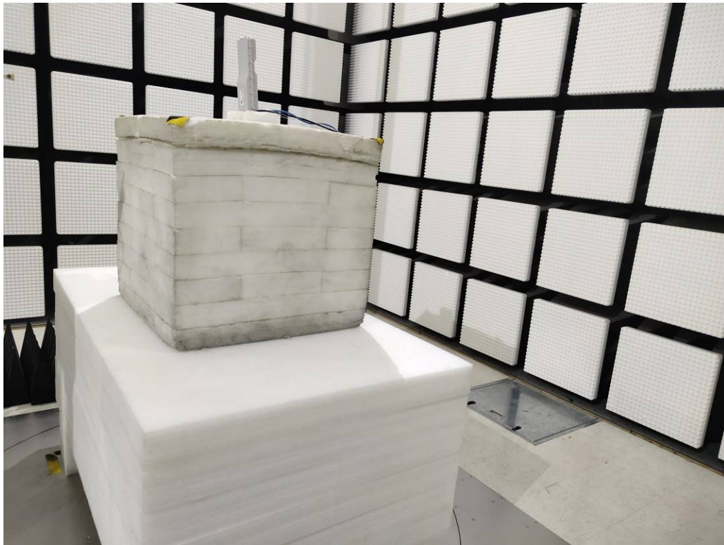
Radiated Emission 90-140GHz View POE
