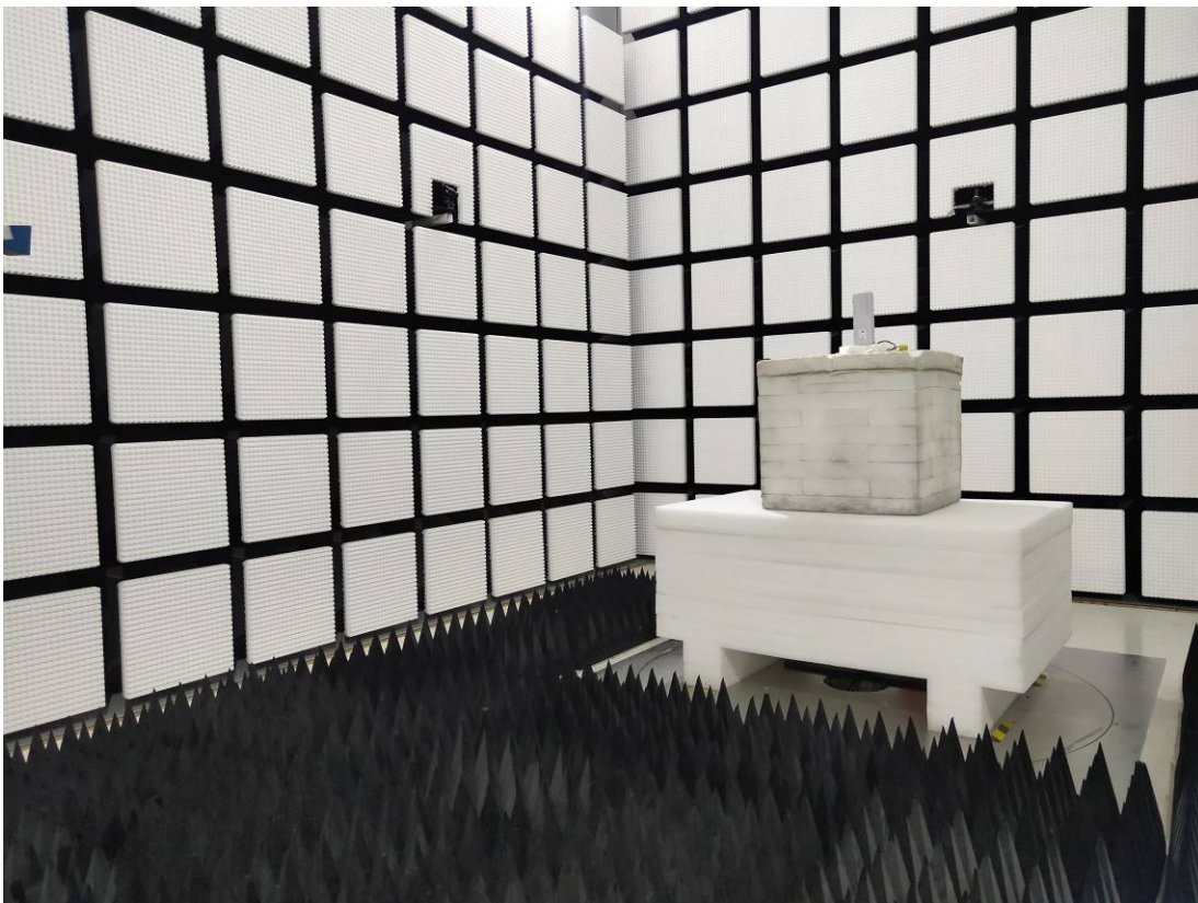
Radiated Emission 18-26.5GHz View POE
