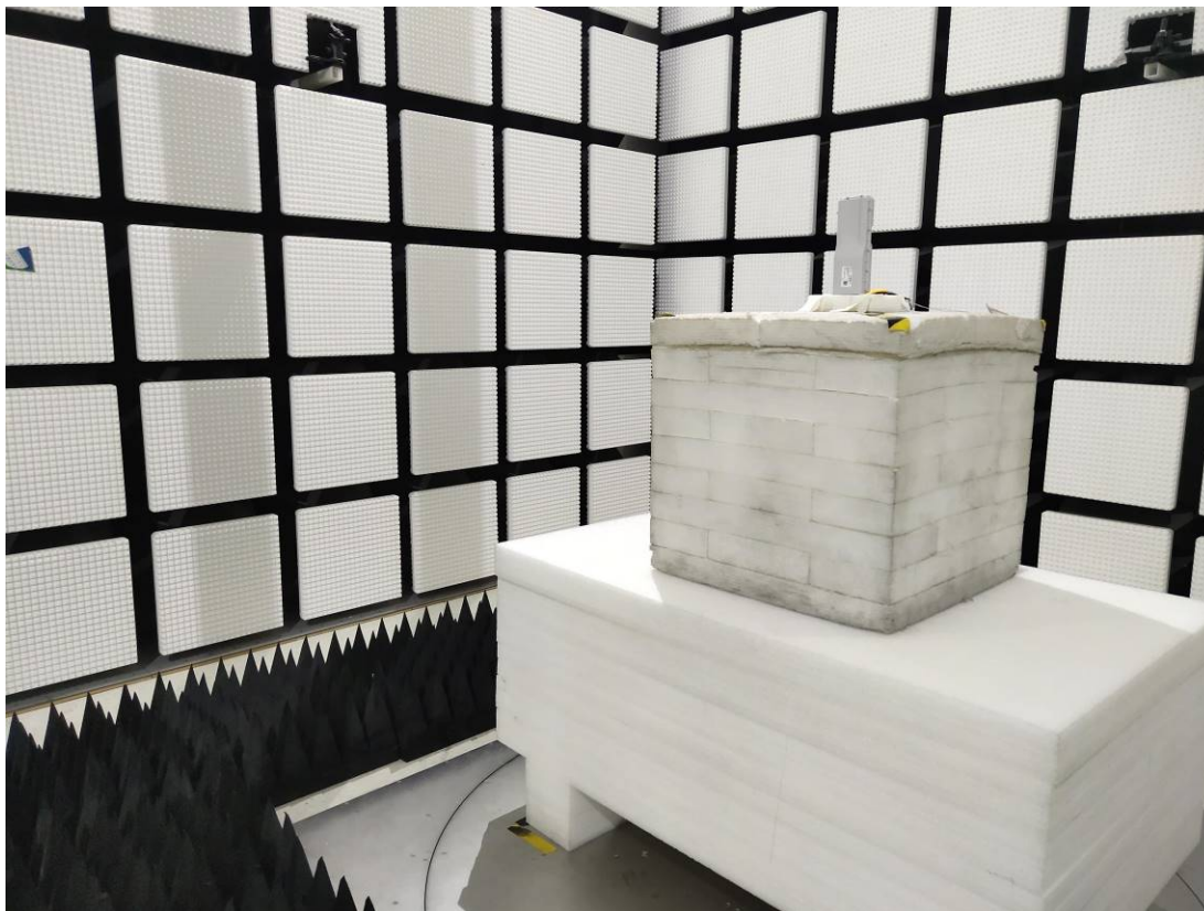
Radiated Emission 40-60GHz View POE
