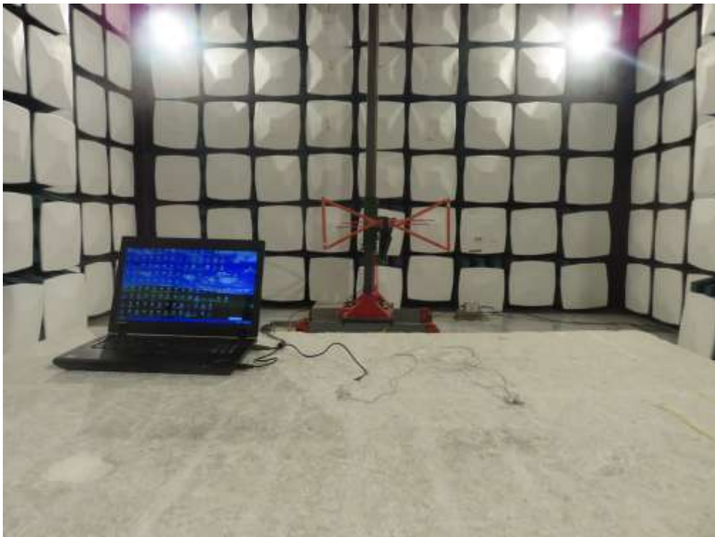
FCC RADIATED EMISSION TEST SETUP
