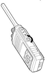
2. Plug the accessory into the accessory connector, and then rotate the screw on the accessory plug clockwise until hand tight.
