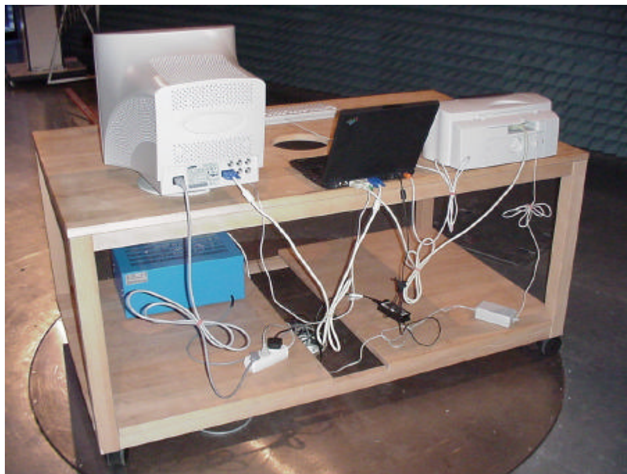
Picture 2 : Setup for radiated emission tests below 1 GHz, rear view
