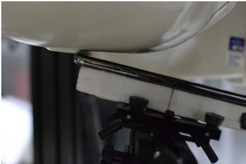
SAR Test Setup Photo 2 – Right Tilt
