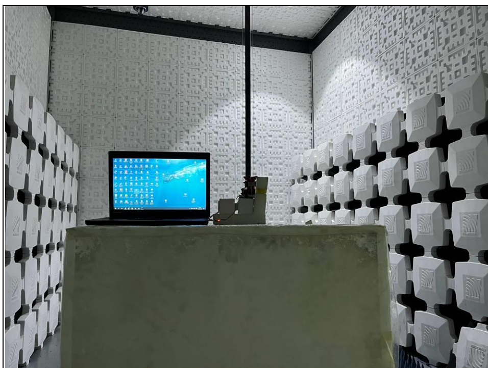
Radiated emission test: Frequency Range< Above 1GHz >
