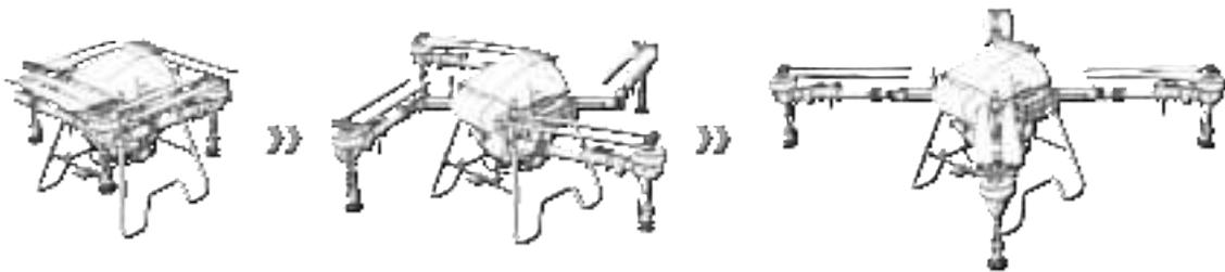
Figure 1-33 Arm Unfolding
