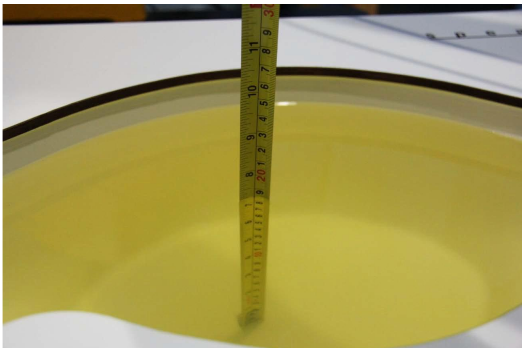
Picture 7-1: Liquid depth in the Flat Phantom(2450MHz)
