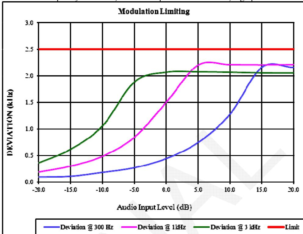
Carrier Frequency: 155MHz, Channel Separation = 12.5 kHz, low power level
