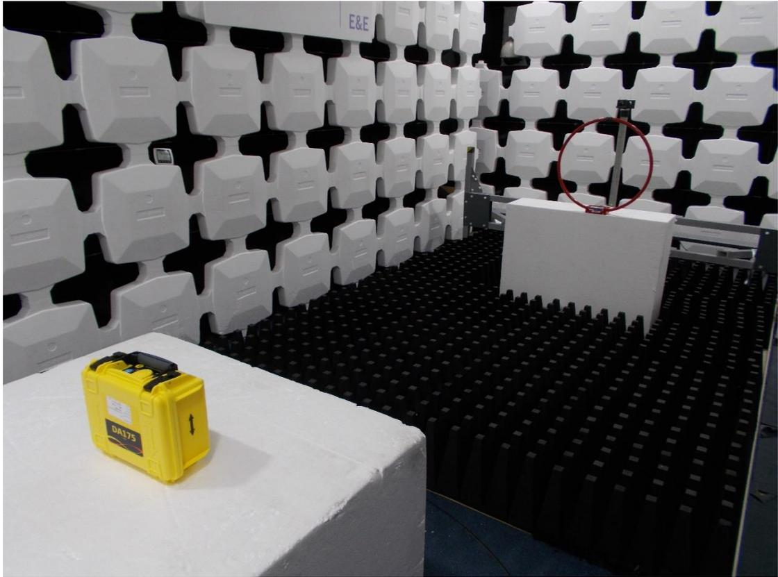
**Radiated emissions 9kHz to 30MHz**
