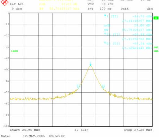
The results: The unit does meet the FCC Part 15 C Section 15.227 requirements.
