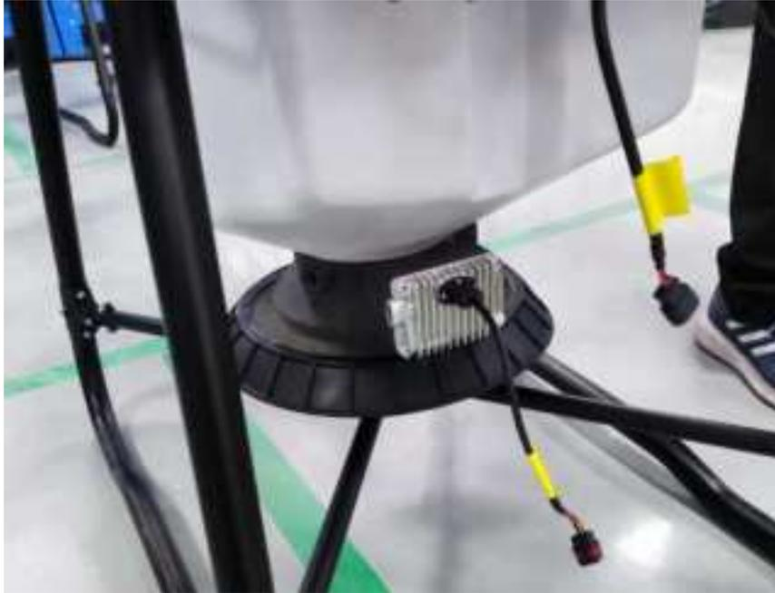
Note: When replacing the Spreading system, please turn off the aircraft power switch first.
