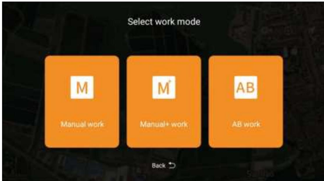
Manual work interface is also the default work interface. This interface can switch other work modes, or call the plot to enter the fully autonomous work mode
