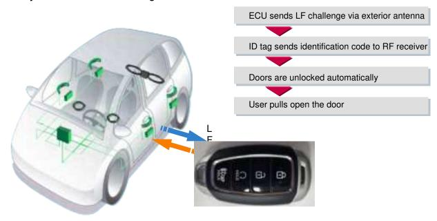
Figure 1: Principle of Communication
