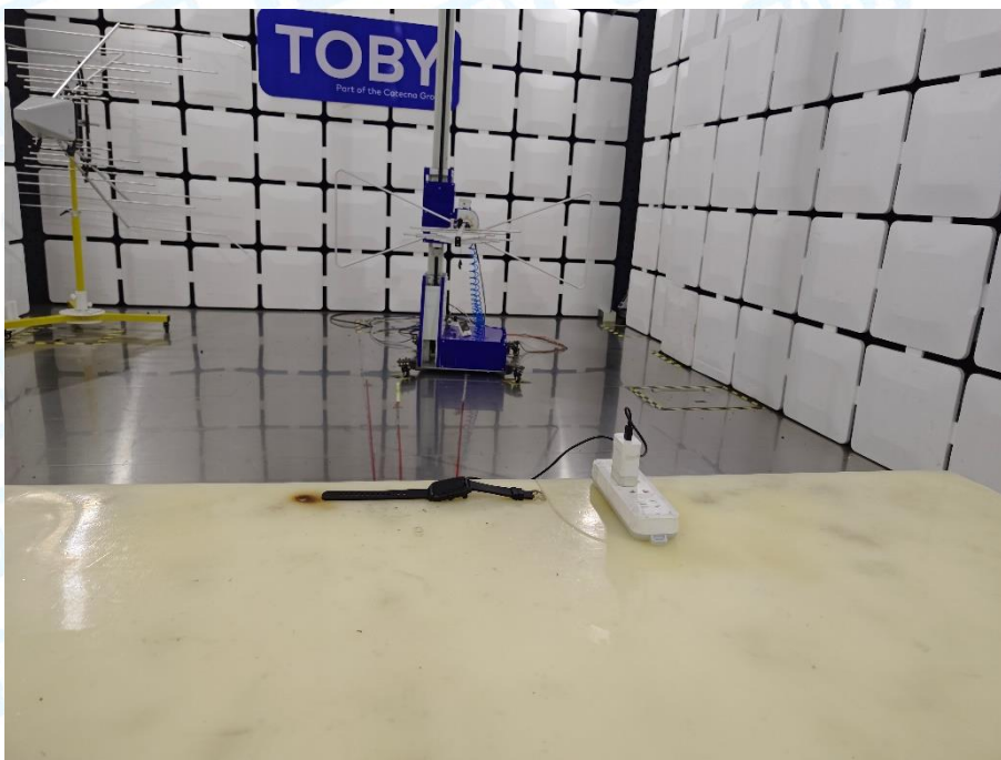
Photo of Setup for Radiated Emission (30MHz~1GHz)
