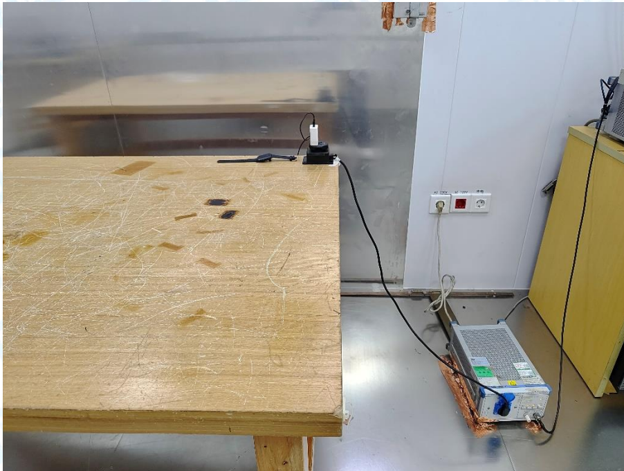
Photo of Setup for Radiated Emission (30MHz~1GHz)
