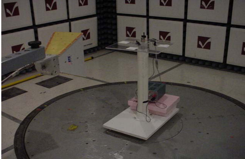
View of the EUT during Radiated Emission Testing in the 3 Meter FCC Listed Chamber, Antenna A
