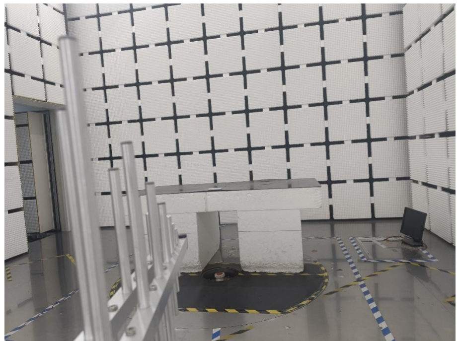
Radiation Emission Test Setup (30MHz to 1GHz)
