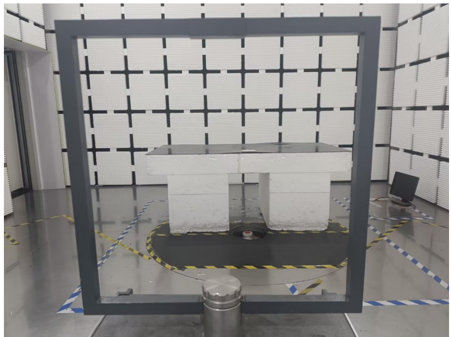
Radiation Emission Test Setup (Below 30MHz)
