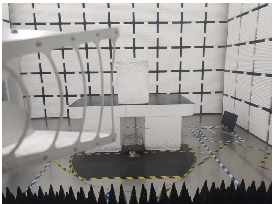
Radiation Emission Test Setup (1GHz to 18GHz)
